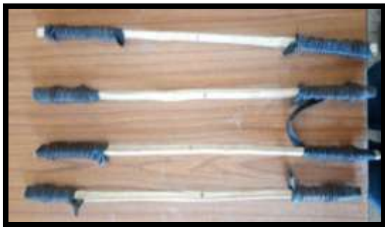
Fig. 4.1: Tensile test specimens of bamboo
