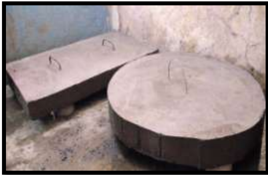
Fig. 5.1: Bamboo ferrocrete manhole covers
